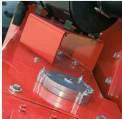
The fine filter in the hydraulic system maintains the oil's performance longer and extends the life span.
