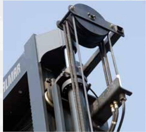
The DCF80-100 has considerably fewer hoses over the mast compared to conventional machines (2 hydraulic hoses and 1 electrical cable). This provides high functional reliability.
